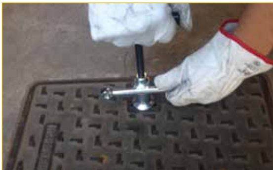
Phase 1: set the hook central bar in the position that can be hooked up by the APS90/APS80.
