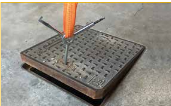
Configuration 4: use in synergy with a choke belt for lifting operations
