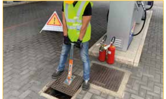
Category 3 ATEX tools suitable for use in places classified ZONE 2.
