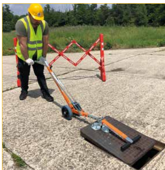
Use 2: opening with wheeled lever APS90.
