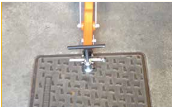
Phase 2: engagement of the lever in the clamp.
