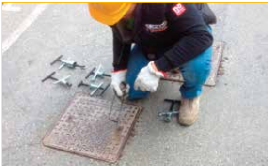
Suitable for mechanical opening of manhole covers.
