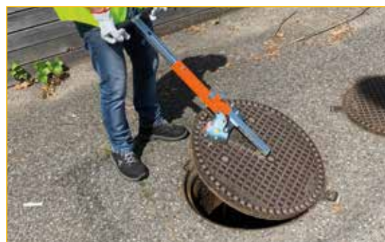
Use 3: Opening with horizontally extended handle bar.
