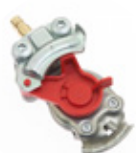
TRUCK COMPRESSED AIR CONNECTION 0.4 kg (0.88 lbs) 529005
