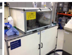
Impulse pressure test stand up to 4000 bar.
