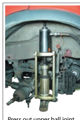
Press out upper ball joint
