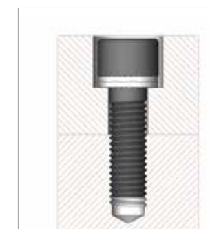
Countersunk socket head bolt secured in position
