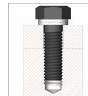
Hexagon bolt secured in a blind hole
